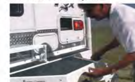
3. Landing folds up, and pin locks it into place
