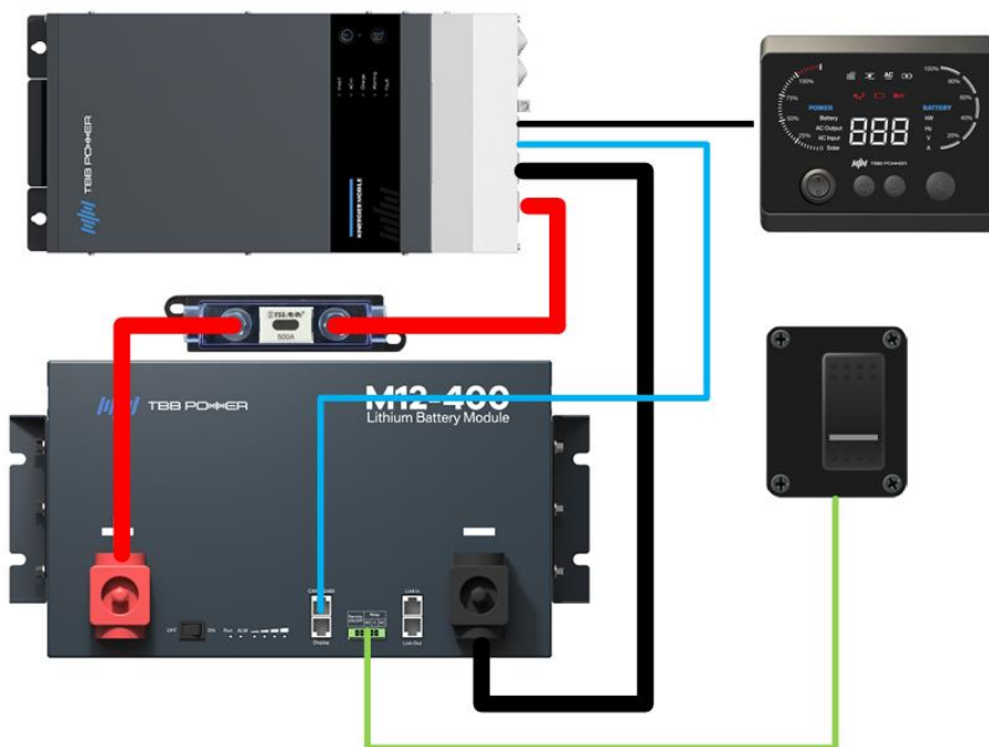
Figure 2-4b Typical wiring diagram 2 (with TBB inverter)
