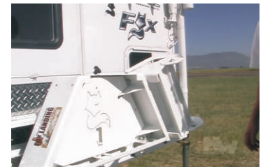
3. Landing folds up, and pin locks it into place
